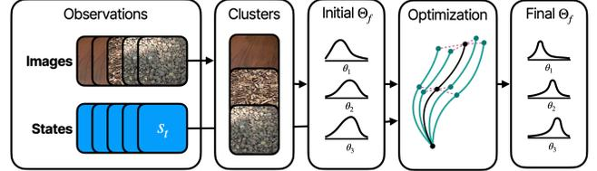
Fig. 1. This figure shows the proposed approach, detailed in Equation (2). Images from our observation are clustered, and an initial guess and the states observed are used to optimize the parameter estimates.
