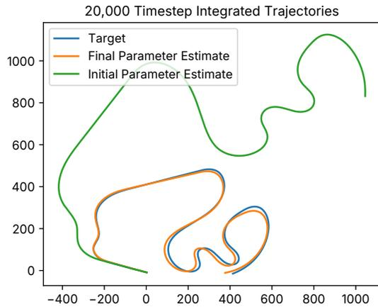
Fig. 2. Numerical simulation results that show the improvement in the parameter estimate. The target data was generated with a multi-body model, and the parameter estimates are generated with a dynamic bicycle model with Pajecka tire forces.
