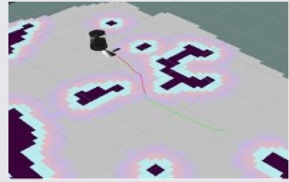
Navigates to within 2 meters of identified piece of trash.
